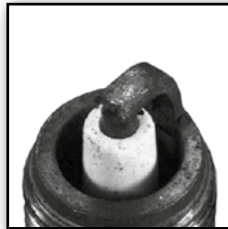
Spark plug has dry deposits
