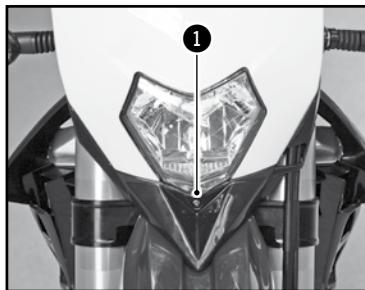
The headlight beam is adjusted with the motorcycle in a state of operation with its driver seated on the saddle.
