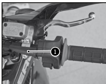
Adjust the throttle cable play at the location shown ① with the adjuster.
