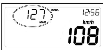
Displays the maximum speed since the last TD reset was performed. (→ p.77)
