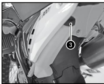
Check the fluid level in the expansion container.
