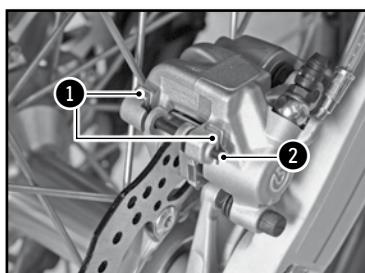
Check that the brake discs are not contaminated with oil or grease. If they are, clean the discs with brake cleaner.
