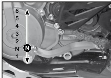
The drawing shows the path of the gear selector for each of the 6 speeds.
