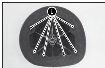
Reposition the filter on its support.
