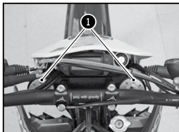
After some time of operation, the air accumulates under pressure in the fork.
