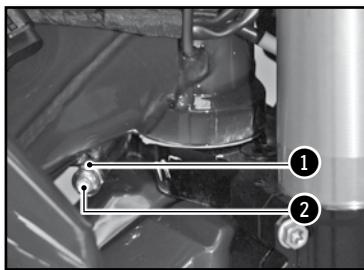
The steering angle can be changed using the set screws located on the bottom of the steering column.
