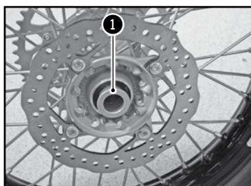
Check that the brake disc is not dirty or contaminated with oil or grease. If it is, clean the disc with brake cleaner.
