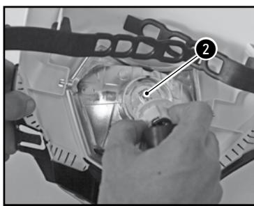
Reinstall the socket with the bulb in the headlight assembly by turning it in a clockwise direction.
