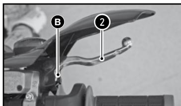
The front brake lever ② is on the right side of the handlebar and has an adjustment screw ③
