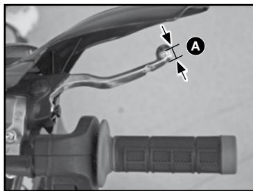
Pull the lever toward the handlebar and check the free play **A**
