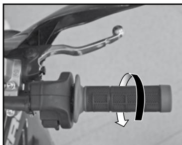
With the handlebars facing straight ahead, check that the throttle twist grip functions properly.
