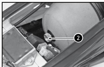
Reinstall the filter and its support by taking special care to make sure it is centered. Refit the knurled screws **2**.
