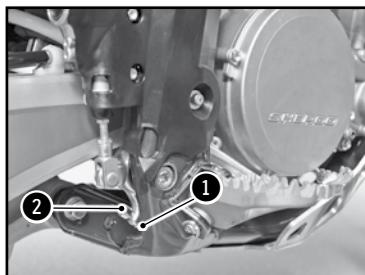
The position of the brake pedal can be adjusted as follows: loosen the lock nut ①, loosen or tighten the screw ② to obtain the desired position.
