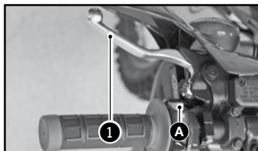
The clutch lever ① is on the left handlebar and has an adjustment screw ②
