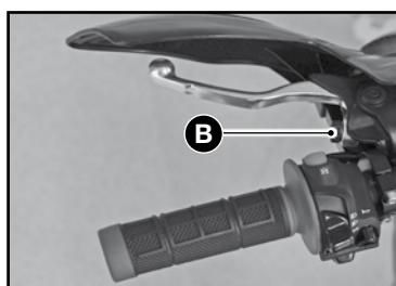
The position of the lever can be adjusted to meet the needs of the rider.
