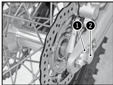
Install the chain tensioner **1** and install the nut **2** but do not tighten.
