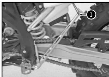
Remove the rubber safety latch ①, using your foot on the shaft unfold it until it supports the weight of the bike.
