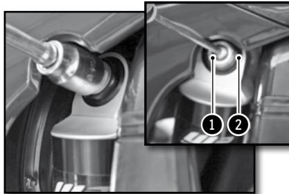
The adjusting screw **1** determines the high speed behaviour of the rear shock (big hits). Turning the screw clockwise increases the hydraulic force (and vice versa).
