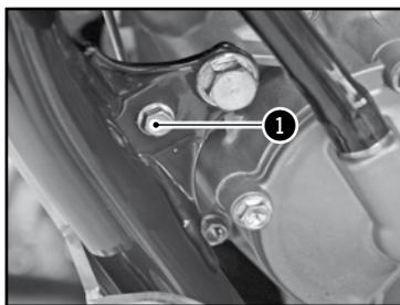
Remove the screws **1** and nuts and remove the bottom plate.
