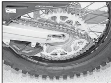
Install the rear wheel in the swing arm and install the axle (grease the axle prior to installation)
