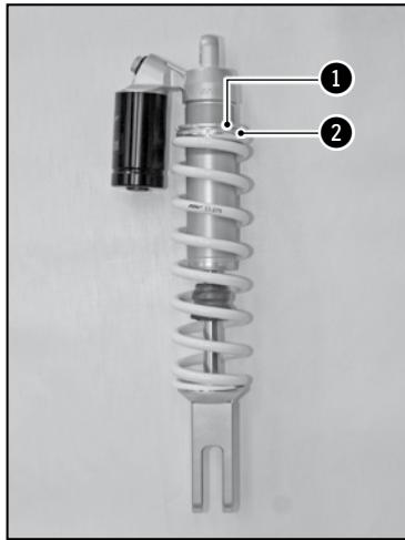
Remove and clean the rear shock unit (☞ p.104).
