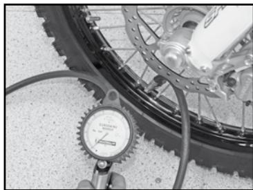
Regularly check the tire pressure with a precision pressure gauge.
