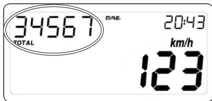
Fig 2 Odometer function - TOTAL
