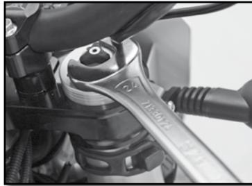
The adjusting nut allows the preload of the Spring to be adjusted. Turning the nut clockwise increases the preload (and vice versa).
