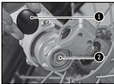
Screws ② determine the behavior of the fork when it is compressed. Turning in the screw-clockwise increases the hydraulic force (and vice versa).
