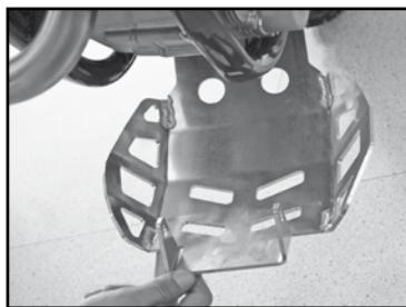
Attach the engine guard at the rear of the frame and rotate upward.
