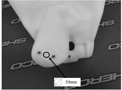
4- Mount the large capacity tank 5185 and the auxiliary tank 7898 and connect the lines # 1 and # 3.
