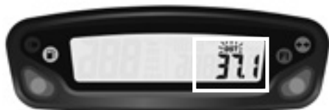
Fig 6 Adjustable trip distance function
