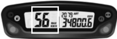
Fig 2 MAX speed function
