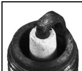
Spark plug has dry deposits
