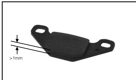
Brake pads in good condition
