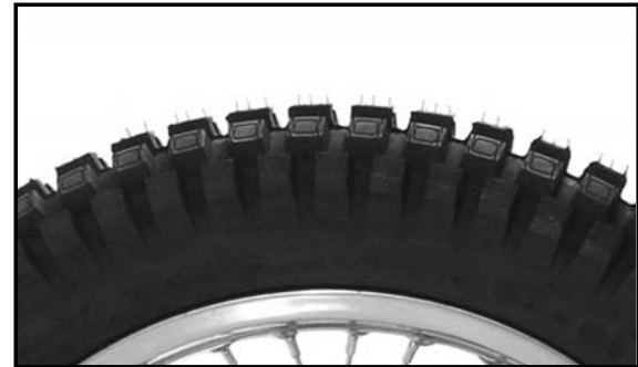
Tyre in good condition
