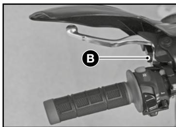
The position of the lever can be adjusted to meet the needs of the rider.
