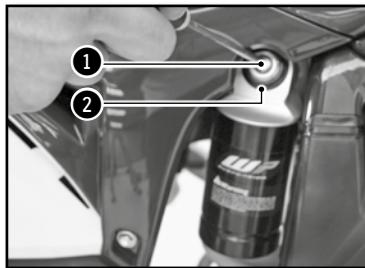
The adjusting screw **1** determines the slow speed behavior of the rear shock (sensitivity). Turning the screw clockwise increases the hydraulic force (and vice versa).
