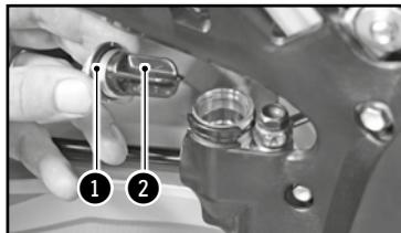
Remove the cap ① with its membrane ②.
