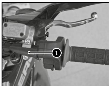
Adjust the throttle cable play at the location shown 1 with the adjuster.
