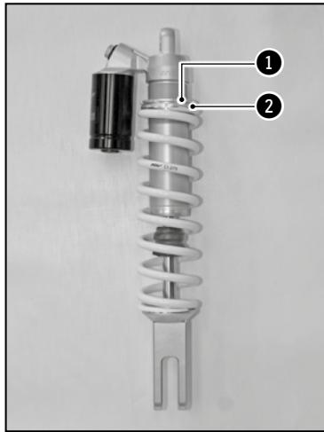
Remove and clean the rear shock unit (☞ p.42).
