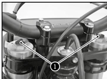
The adjusting screws ① determine the behavior of the fork when it rebounds. Turning the screws clockwise increases the hydraulic force (and vice versa).
