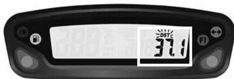
**Fig 6 Adjustable trip distance function**
