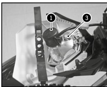
Remove the headlight housing assembly (☞ p.116)
