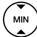
If the level is below the MIN mark, top up the brake fluid according to the instructions below.
