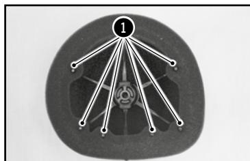
Reposition the filter on its support.
