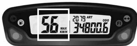
**Fig 2 MAX speed function**
