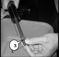
Place the suspension arm vertically and pour 250cc of new oil inside.
