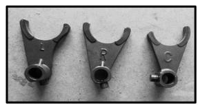
• Insert the forks **[2]** on the gears and mount the gearbox / fork assembly in the crankcase.
