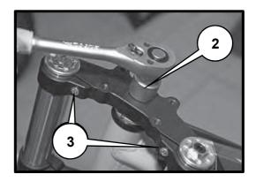
Loosen the steering column lock nut [4] and its dust cover, then separate the complete Fork of the frame
