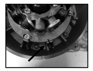
• Remove the three M6 screws **[1]** for fixing the stator then the two M5 screws **[2]** for fixing the pick-up sensor and take out the assembly.
