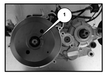
• Fit the extractor **[2]** reference R075 and tear off the magnetic flywheel **[3]**.
