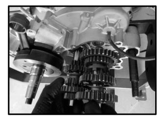
WARNING When removing, take care to identify the location of the washers at the end of the shaft.
