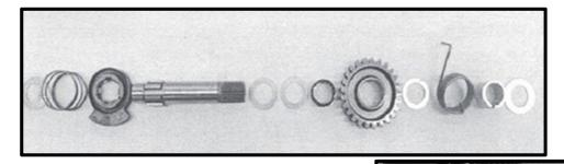
• Fit the shaft [1] and its spring so that the slide [2] comes against the stop of the housing [3].
