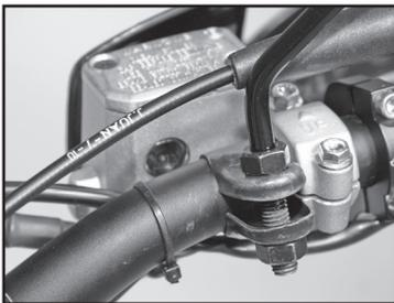
Make sure that the reservoir is in a horizontal position.
