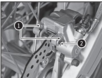
Check that the brake discs are not contaminated with oil or grease. In they are, clean the discs with brake cleaner.
