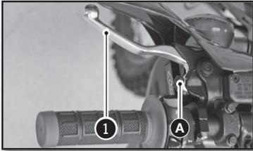
The clutch lever **1** is on the left handlebar and has an adjustment screw **A**
