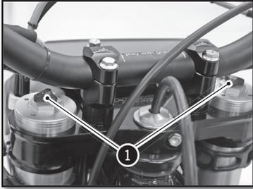
The adjusting screws ❶ determine the behavior of the fork when it rebounds. Turning the screws clockwise increases the hydraulic force (and vice versa).
