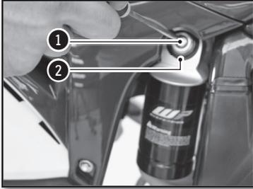
The adjusting screw ① determines the slow speed behavior of the rear shock (sensitivity). Turning the screw clockwise increases the hydraulic force (and vice versa).
