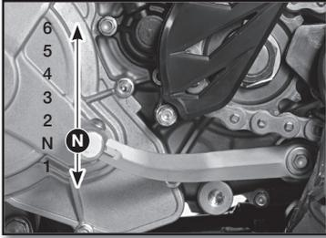
The drawing shows the path of the gear selector for each of the 6 speeds.
