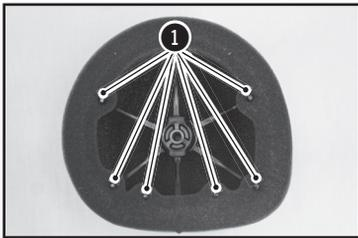
Reposition the filter on its support.
