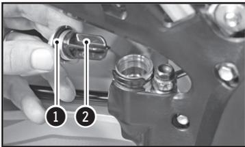
Remove the cap ① with its membrane ②.
