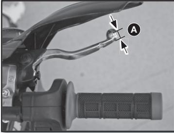
Pull the lever toward the handlebar and check the free play **A**
