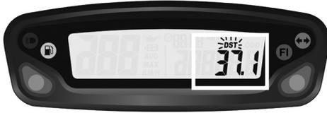
Fig 6 Adjustable trip distance function
