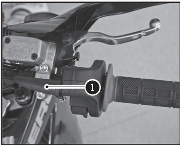
Adjust the throttle cable play at the location shown ❶ with the adjuster.
