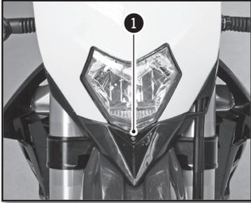
The headlight beam is adjusted with the motorcycle in a state of operation with its driver seated on the saddle.
