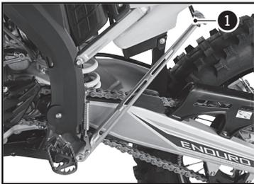
Remove the rubber safety latch 1, using your foot on the shaft unfold it until it supports the weight of the bike.
