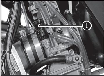
The choke lever **1** is fitted on the left side of the carburetor.
