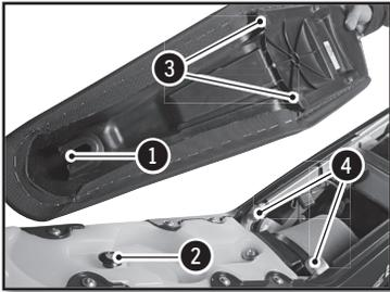
Install the saddle by sliding it forward, making sure that the slot **1** in the seat pan engages the post **2** in the reservoir. The three notches in the saddle must pass through the tabs on the subframe **4** that are provided for this purpose.
