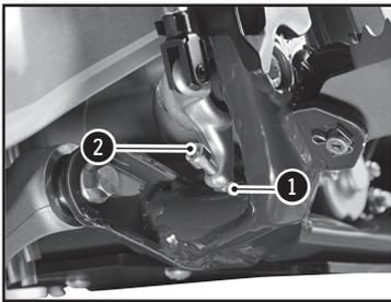
The position of the brake pedal can be adjusted as follows: loosen the lock nut ① loosen or tighten the screw ② to obtain the desired position.
