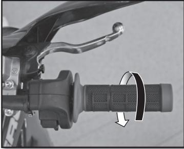
With the handlebars facing straight ahead, check that the throttle twist grip functions properly.
