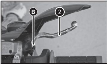
The front brake lever **2** is on the right side of the handlebar and has an adjustment screw **B**
