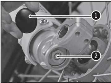
Screws **2** determine the behavior of the fork when it is compressed. Turning in the screw clockwise increases the hydraulic force (and vice versa).
