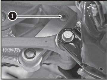
The adjusting screw **1** determines the Shock rebound behavior. Turning the screw clockwise increases the hydraulic force (and vice versa).
