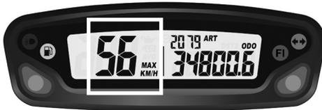
Fig 2 MAX speed function
