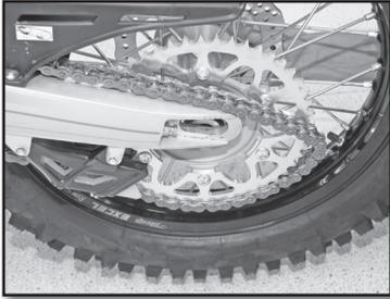
Install the rear wheel in the swing arm and install the axle (grease the axle prior to installation)
