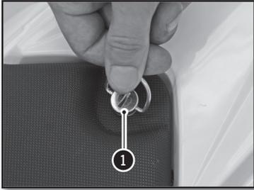
Turn the Dzeus fastener **1** a quarter turn counterclockwise to release the saddle.
