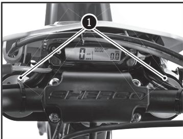
After some time of operation, the air accumulates under pressure in the fork.
